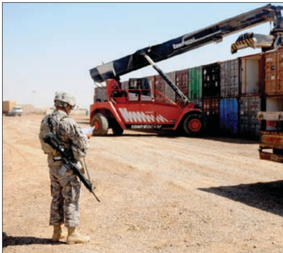
A Soldier looks on as a rough terrain container handler picks up an empty container and loads it on a flatbed truck at the Receiving and Shipping Point yard at Joint Base Balad, Iraq. The CRSP will be relocated to an expanded location, tripling its cargo capacity.
