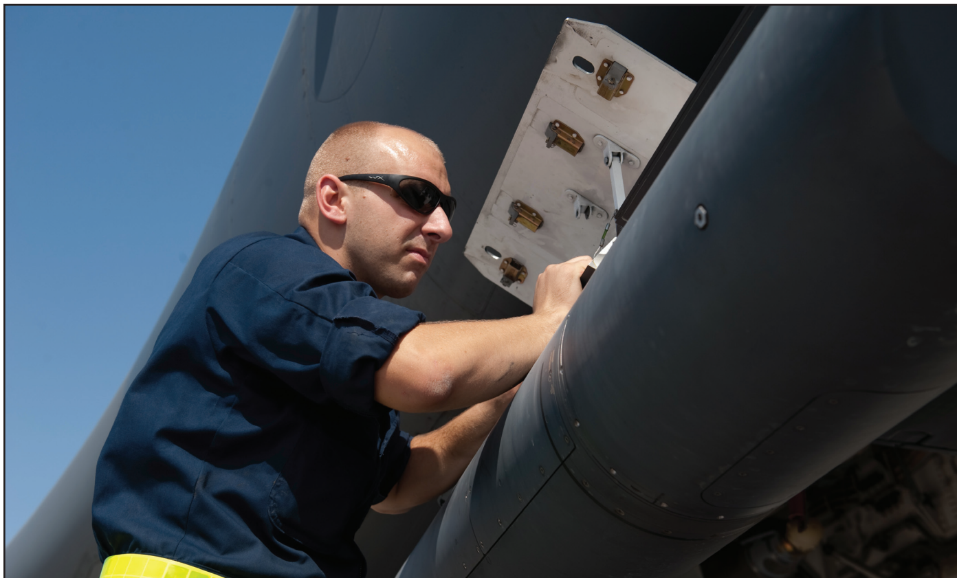
Senior Airman Brad Emerson, 37th Aircraft Maintenance Unit offensive aviation systems technician, checks for proper installation of the Sniper Advanced Targeting Pod on a B-1B Lancer, Nov. 15, in Southwest Asia. Airman Emerson is deployed from Ellsworth Air Force Base, S.D. in support of operations Iraqi and Enduring Freedom.
