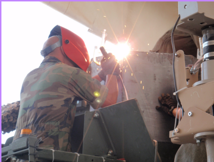
Sgt. Billy McClesky, from the 702nd Brigade Support Battalion, welds “pope glass” onto a Stryker. McClesky serves on the Combat Repair Team (CRT) that directly supports 1st Battalion, 38th Infantry Regiment on Camp Liberty. (Courtesy photo by U.S. Army)
