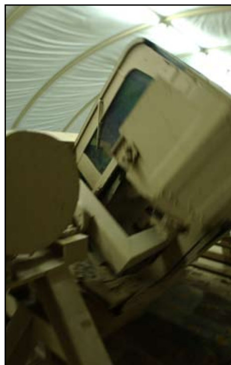
A HEAT trainer spins, simulating a vehicle rollover. Camp Buehring's training village has six of these systems to train servicemembers on how to react to a vehicle rollover.
