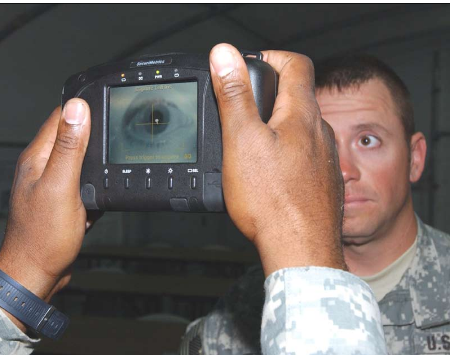
Soldier gets a picture of his retina taken during a Biometrics training class at Camp Buehring. Biometrics enables Soldiers to keep track of detected terrorists and quickens the identification process.
