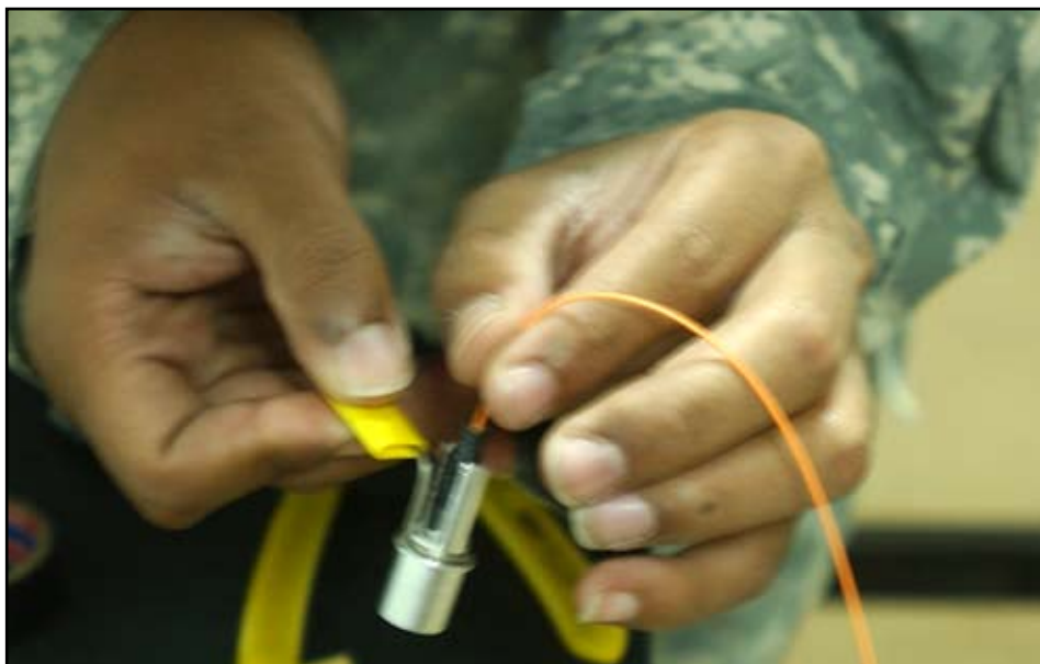
A student of the fiber optics class at the Signal University on Camp Arifjan, Kuwait, threads the hair-thin glass through a small hole.
