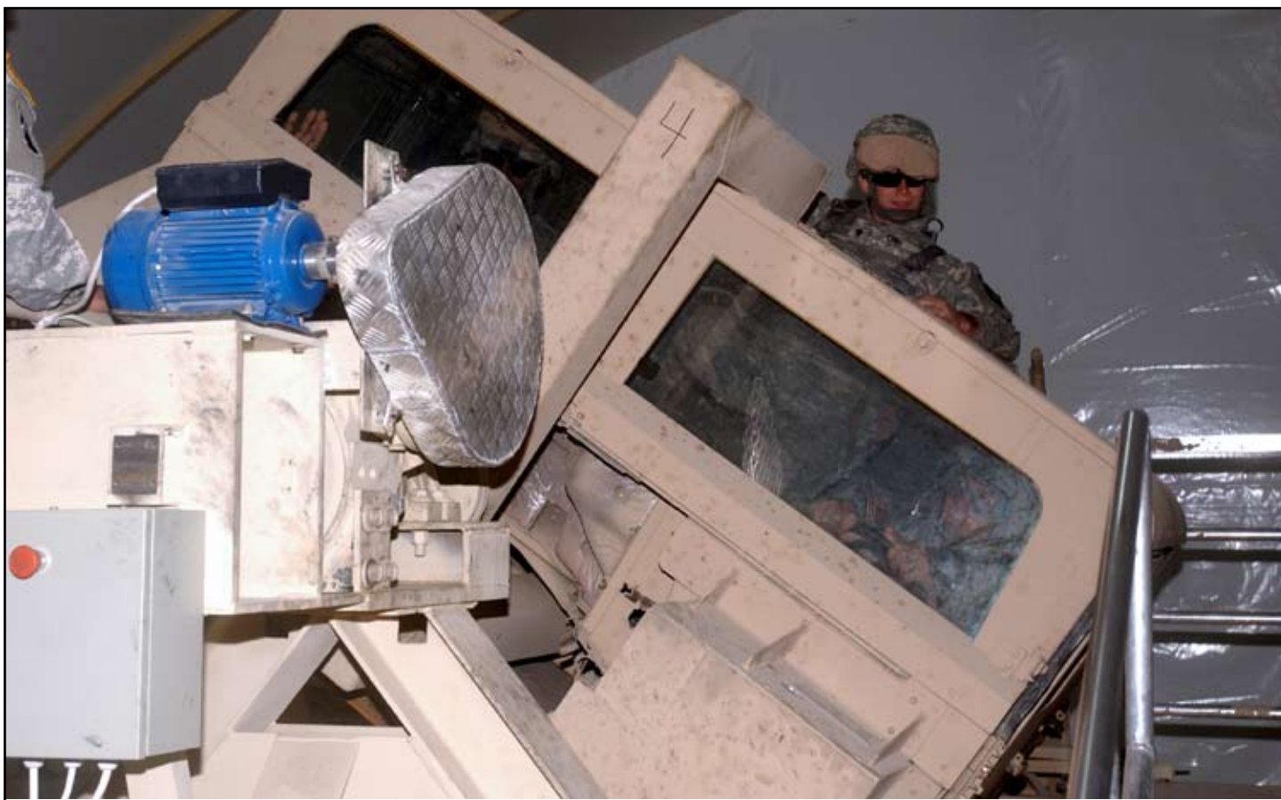
A Soldier goes through the HEAT at the training site on Camp Buehring, Kuwait. The goal of the simulator is to teach service-members how to escape the Humvee should an accident occur. More HEATs are being delivered throughout Kuwait.
