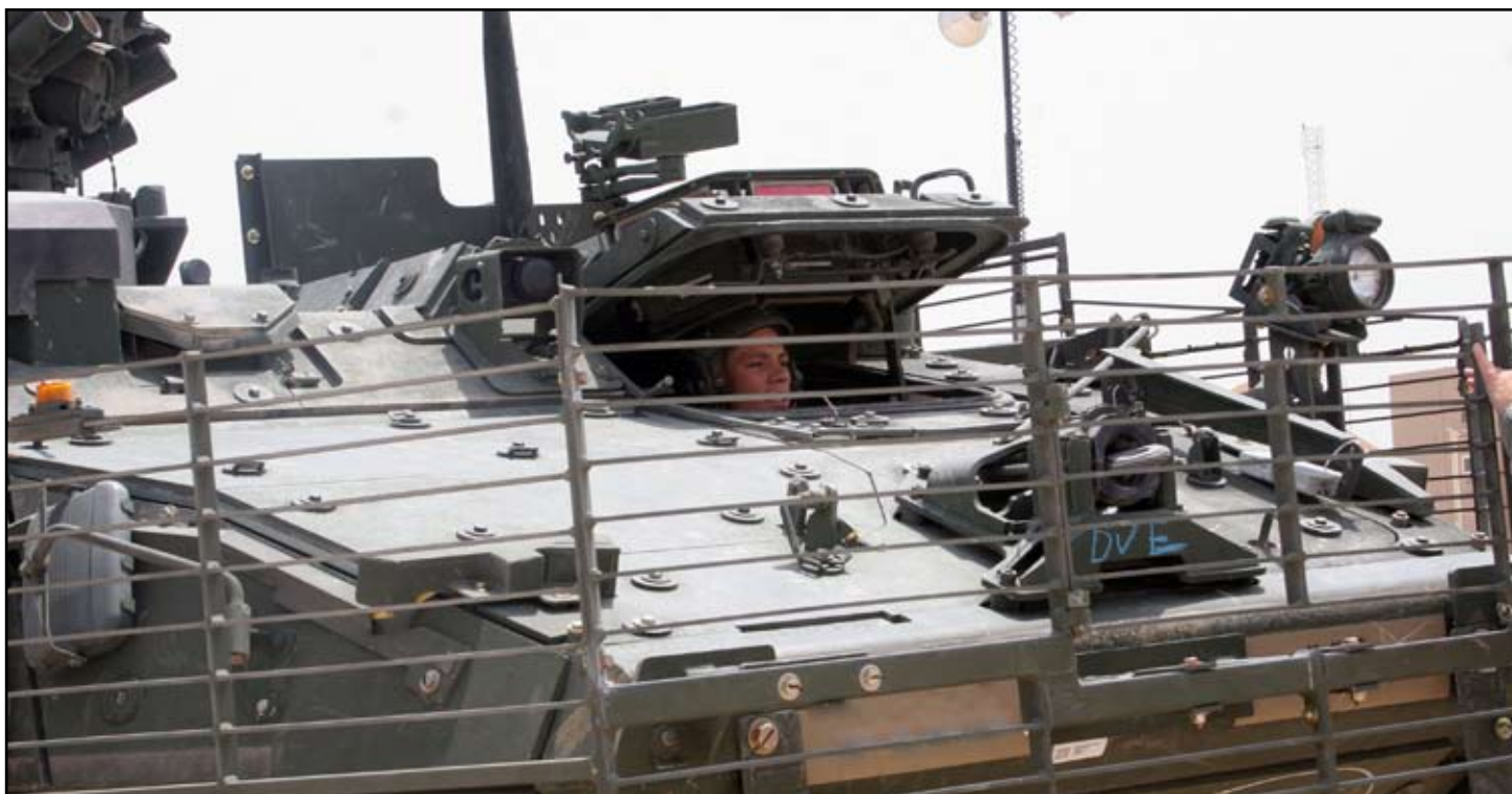
Pfc. Michael Burgner, 2nd SCR, a native of Oswego, Ill., drives a Stryker equipped with the new Remote Weapon System and the anti-RPG Slat Armor at Camp Arifjan, Kuwait. The equipment upgrades were performed using Third Army/U.S. Army Central facilities.
