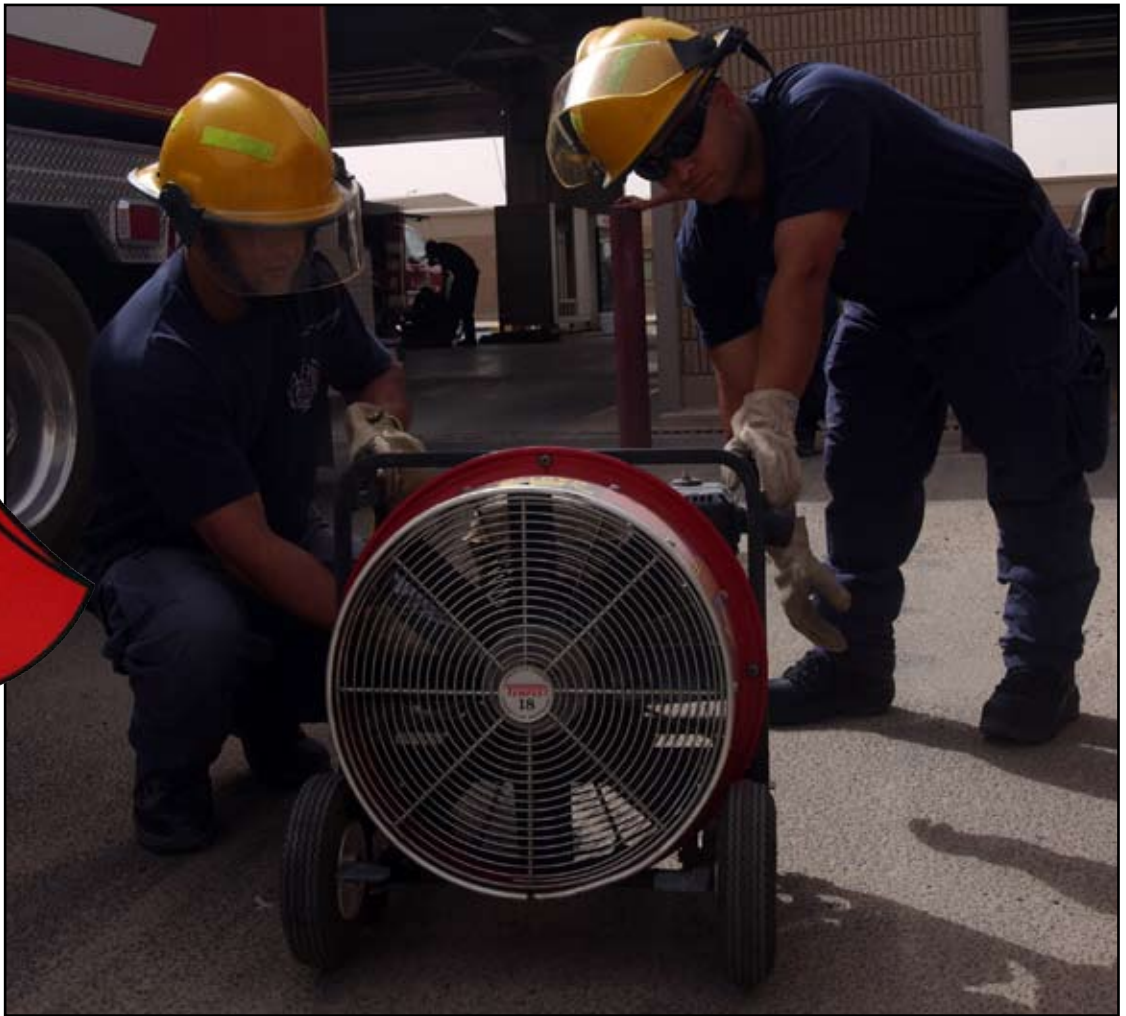
Firefighters Manoj Thakuri, left, and Dinesh Panta conduct a functions check on a positive pressure fan. The fan is used by firefighters to ventilate smoke out of a building by forcing air through it.
