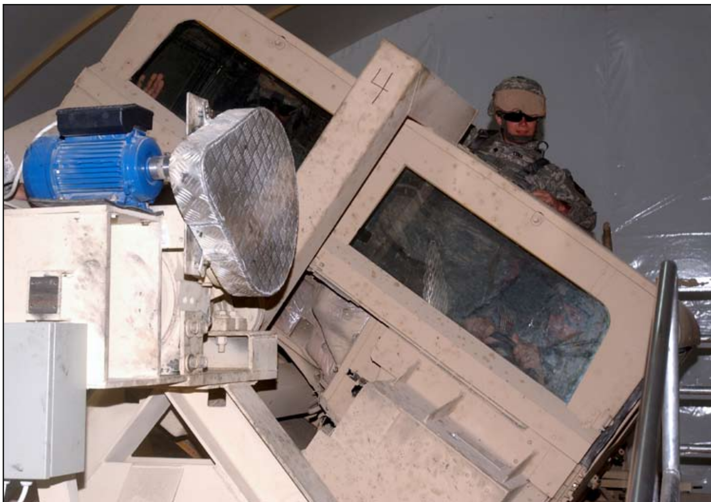
Spc. Joshua Coke, Headquarters and Headquarters Company 12th Combat Aviation Brigade, sits in the turret seat as the humvee simulator simulates a 25 degree angle to the right. The training is designed to teach servicemembers how to react to a humvee rollover accident.
