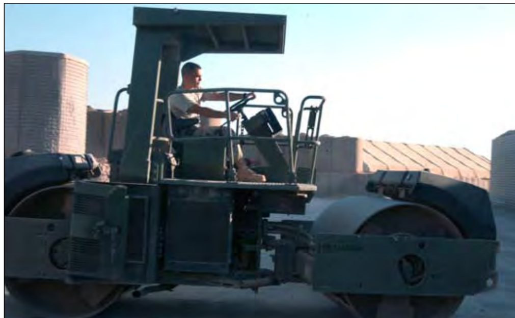
Senior Airman William Cravener operates a steel wheel roller Nov. 3 at Balad Air Base, Iraq. Airman Cravener is a 332nd Expeditionary Civil Engineer Squadron pavements and equipment journeyman deployed from Spangdahlem Air Base, Germany.
