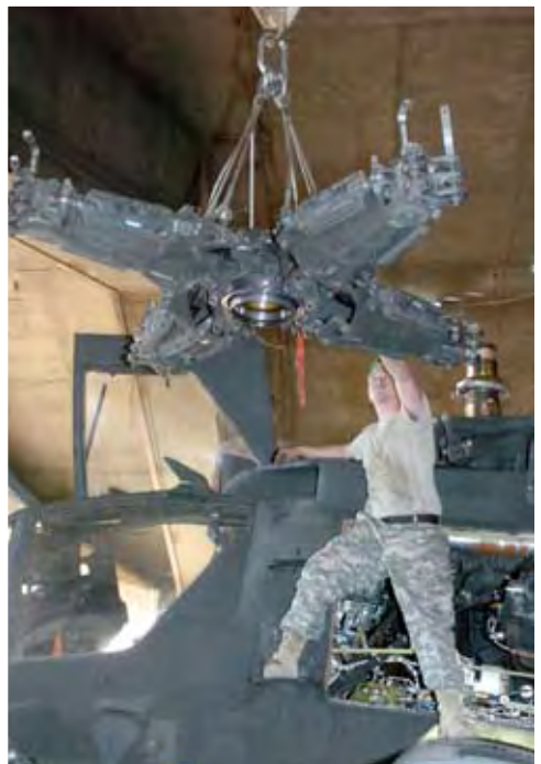
Sgt. Labon Hassett, Company D, 1st Battalion, 149th Aviation Regiment (Attack), from Grants Pass, Ore., helps guide an Apaches' main rotor head suspended by a crane. The rotor will be fully torn down and inspected while the helicopter gets a new one.
