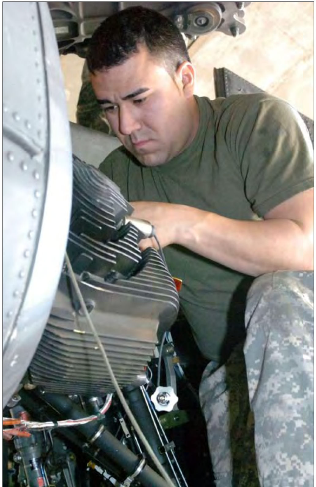
Spc. Daniel Acevedo, B Company, 1st Battalion, 449th Aviation Support Battalion, from Houston, checks all the wires inside an Apache helicopter's nose gear box.
