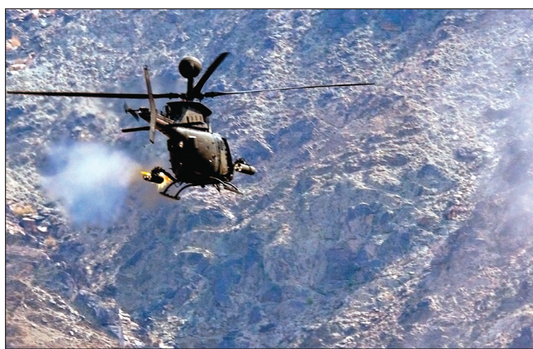
An OH-58D Kiowa Warrior from Task Force Saber, 82nd Combat Aviation Brigade, fires a 2.75-inch rocket at a mountainside during a test flight in eastern Afghanistan. (U.S. Army photo/Sgt. 1st Class Eric Pahon)
