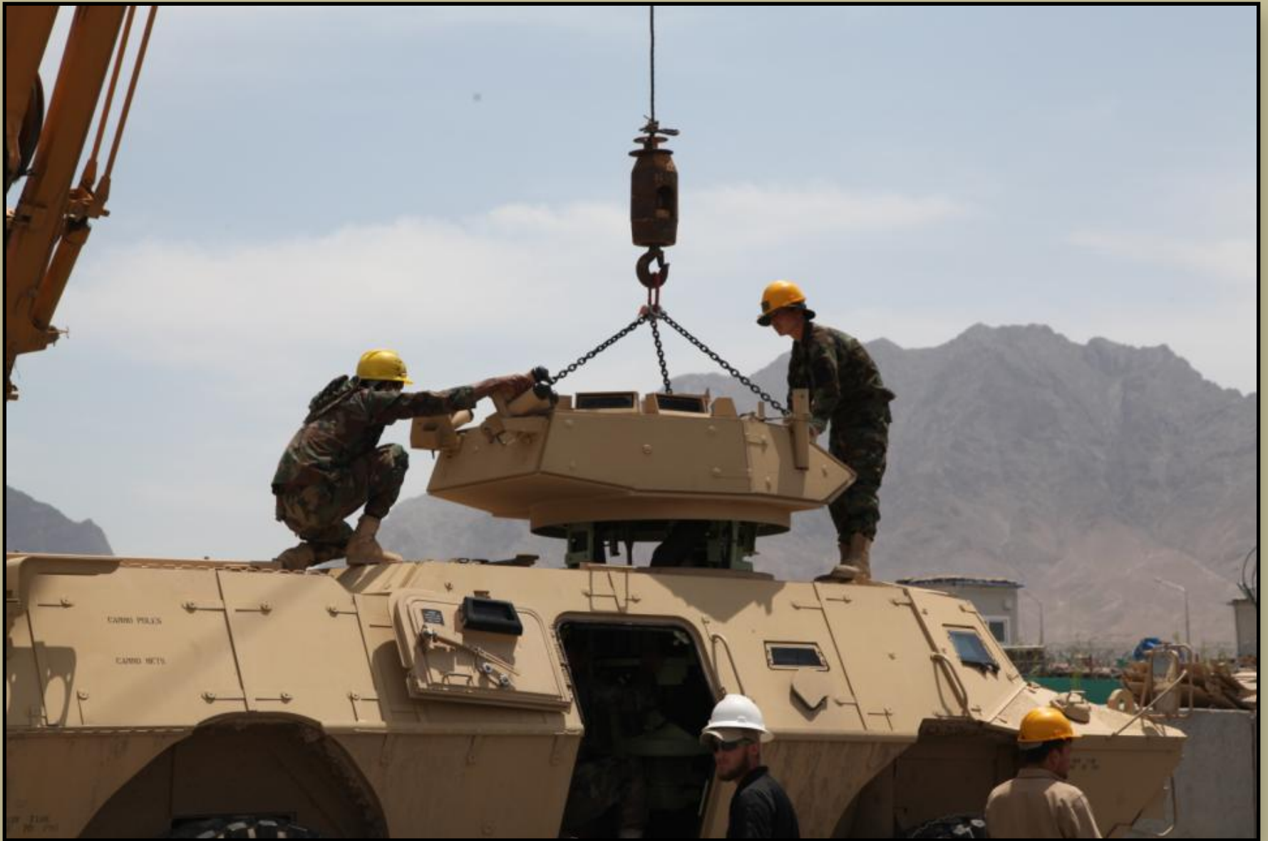
Afghan National Army (ANA) students remove the turret on a Mobile Strike Force Vehicle for maintenance on a Mobile Strike Force Vehicle at the ANA Armored Branch School in Kabul province, Afghanistan, May 7, 2013. These ANA students are fuel level maintenance mechanics in their 3rd of 12 weeks of maintenance training. (U.S. Army photo by Sgt. Kent Redmond/Released)
