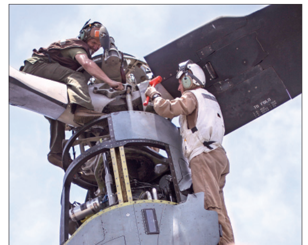
Marines prepare to dismantle the rotor of a MV-22 Osprey on the flight deck of the USS Kearsarge May 4.
