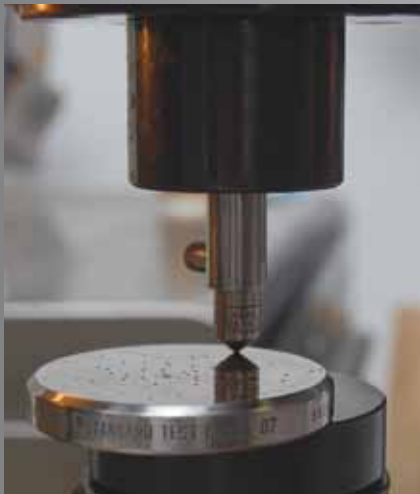
A part is tested for hardness during a destructive test.
