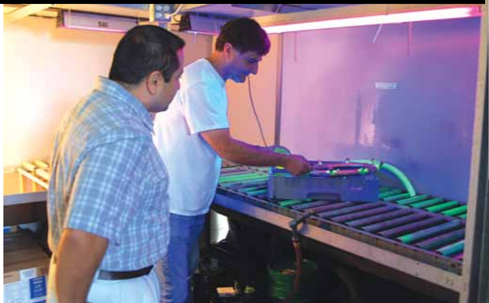
Enrique Rodriguez, DCMA quality assurance specialist, verifies a liquid penetrant inspection is performed as required per contractual guidelines.
