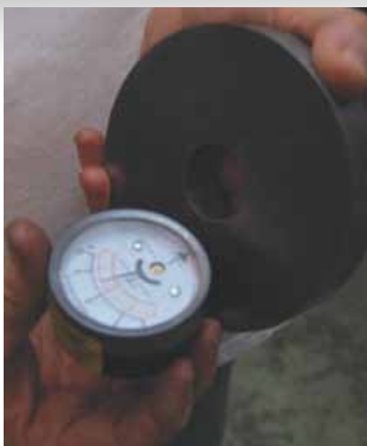
A gauge is used to ensure parts are magnetized prior to a magnetic particle inspection.
