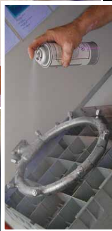
A developer is applied to a part during a liquid penetrant inspection.
