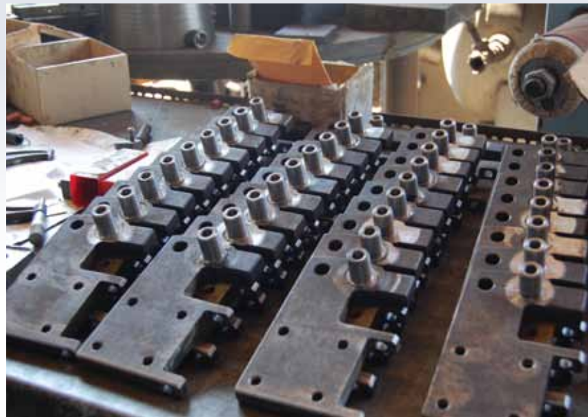
Machined parts await final touches before being ready for shipment. DCMA quality assurance specialists randomly select parts from the group for inspection and to test tolerances. (Photos by Matthew Montgomery, DCMA Public Affairs)
