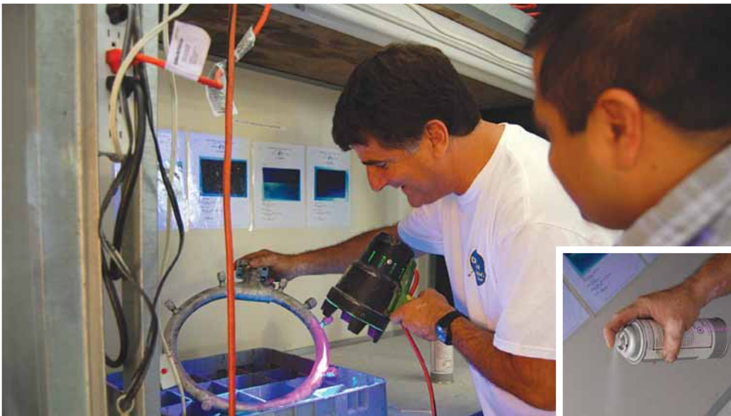
Enrique Rodriguez, DCMA quality assurance specialist, verifies a liquid penetrant inspection is performed as required per contractual guidelines.
