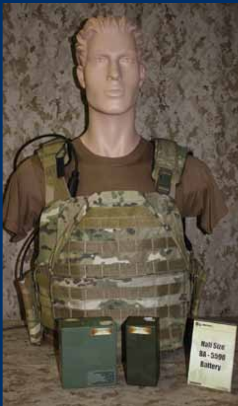
The Half-Sized BA-5590 is an alternate solution to the standard BA-5590. This new half-sized primary battery provides similar performance and runtime in half the weight and volume as the BA-5590. (U.S. Army photo)
