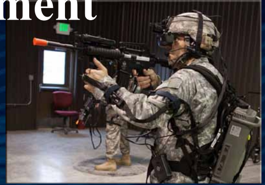
Capt. Marcus Long, 157 th Infantry Brigade operations officer, First Army Division East, takes advantage of the Dismounted Soldier Training System. The helmet-mounted display provides a realistic virtual training platform programmable for any theater of operations while sensors on the body harness capture the Soldiers movements. The natural movements are then translated to control the Soldier’s avatar within the simulation.
