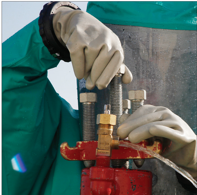
A CBRN defense specialist with MWHS-2 tightens a release cylinder hood while attempting to stop leaks as part of a HAZMAT technician certification course here. Before participating in the course, the Marines completed the HAZMAT operations and awareness prerequisite.
