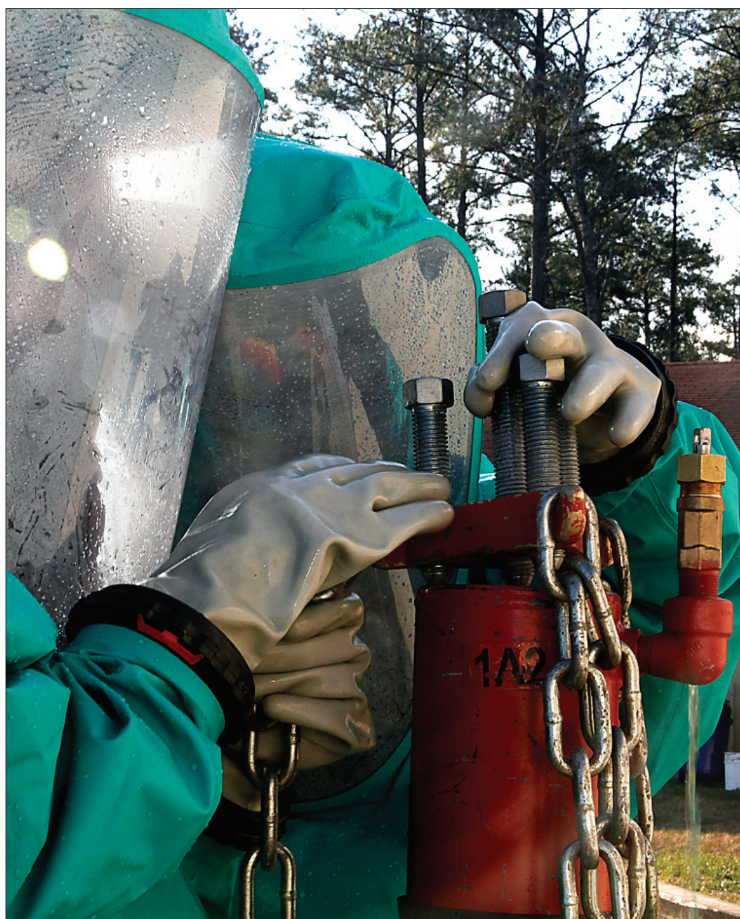
CBRN defense specialists with MWHS-2 use chains to secure a release cylinder hood.
