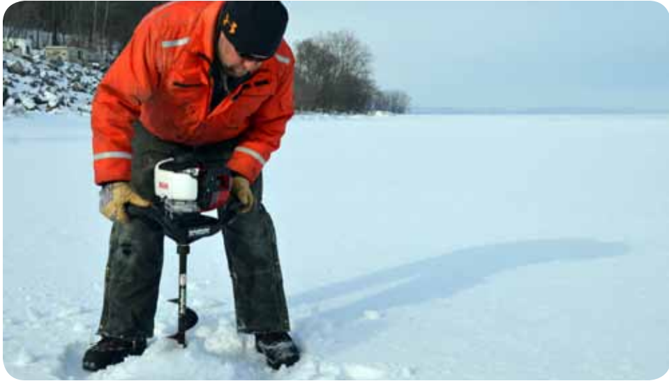
Bill Chelmowski, operations, uses an ice auger to drill a hole on Lake Pepin, near Wabasha, Minn., Feb. 13, during the first Mississippi River ice surveys of the year.
