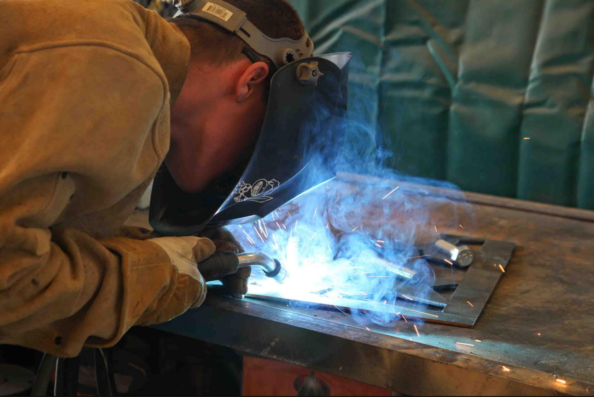
U.S. Army Pfc. Nicholas Direnzo, a wheeled vehicle mechanic with Fox Company, 3rd Battalion (Airborne), 509th Infantry Regiment, Task Force 4-25, welds a bolt to a custom shelf bracket on Forward Operating Base Gardez, Paktia province, Afghanistan, Aug. 25, 2012. (U.S. Army photo by Sgt. Kimberly Trumbull / Released)
