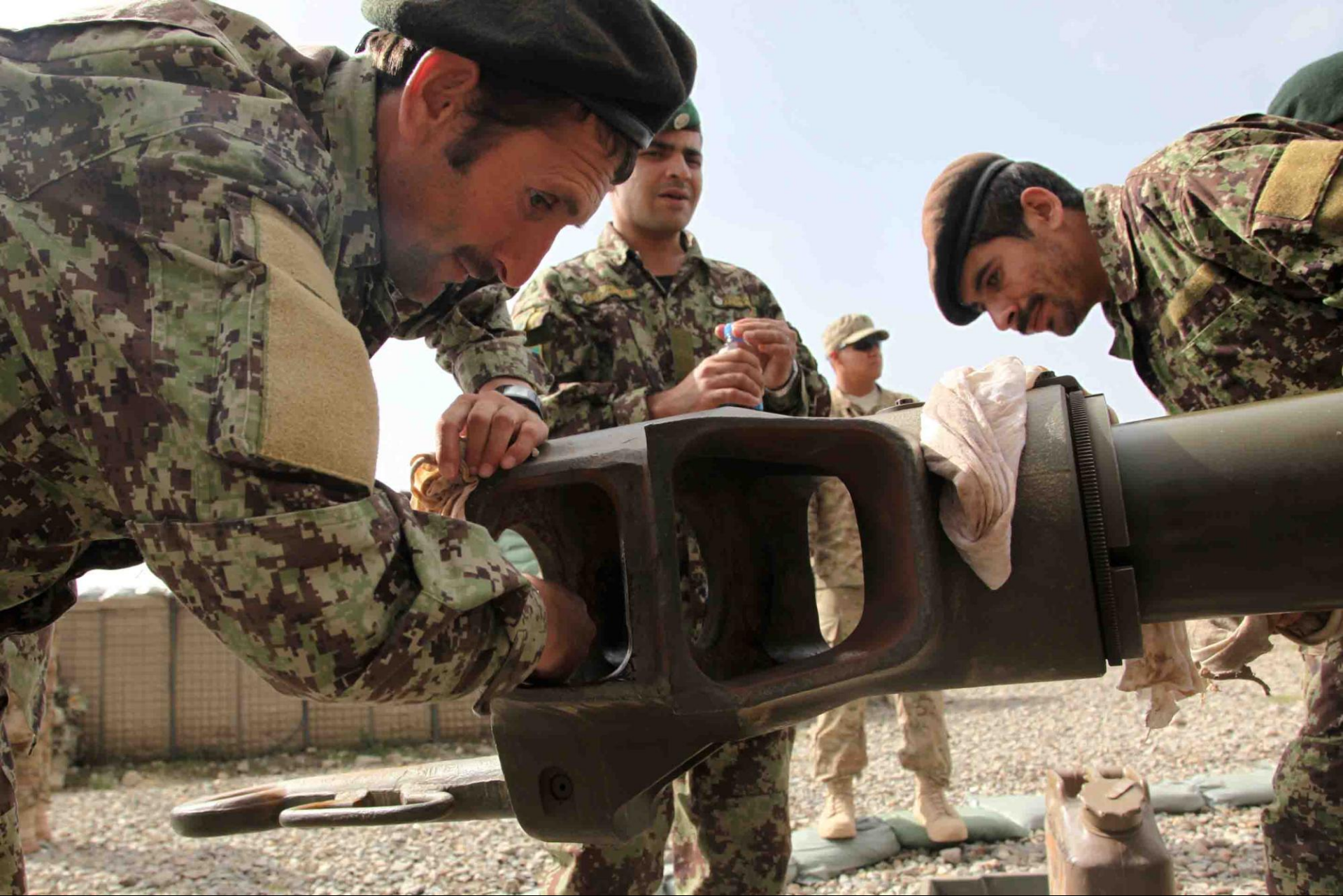
An Afghan National Army (ANA) soldier rubs oil onto unpainted surfaces of a D-30 122 mm howitzer on Camp Clark, Khost province, Afghanistan, Sept. 17, 2012. U.S. Soldiers with Bravo Battery, 2nd Battalion, 377th Parachute Field Artillery Regiment, Task Force 4-25, trained and certified the ANA soldiers on the D-30. (U.S. Army photo by Sgt. Kimberly Trumbull/Released)
