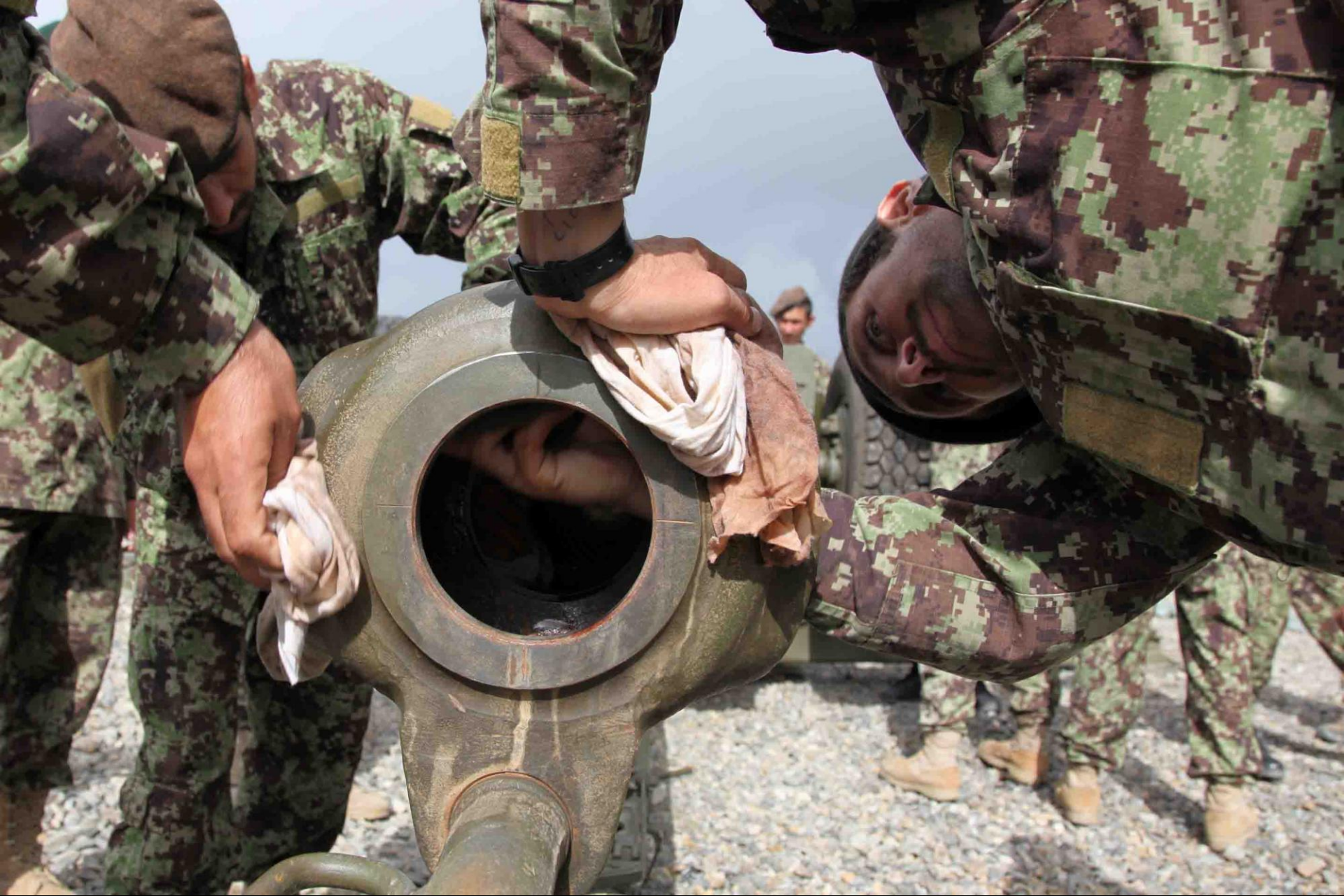
Afghan National Army (ANA) soldiers rub oil onto unpainted surfaces of a D-30 122 mm howitzer on Camp Clark, Khost province, Afghanistan, Sept. 17, 2012. U.S. Soldiers with Bravo Battery, 2nd Battalion, 377th Parachute Field Artillery Regiment, Task Force 4-25, trained and certified the ANA soldiers on the D-30. (U.S. Army photo by Sgt. Kimberly Trumbull/Released)
