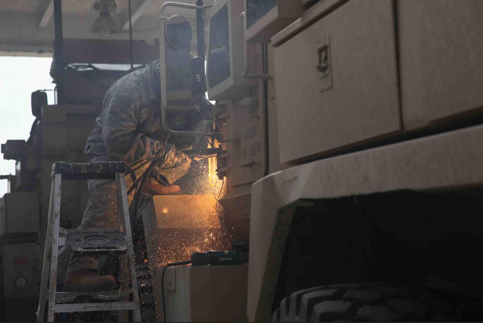
Saji Thomas, a force protection field service representative welder, repairs a door hinge on a mine-resistant, ambush-protected vehicle on Forward Operating Base Salerno, Khost province, Afghanistan, Aug. 10, 2012. (U.S. Army photo by Sgt. Kimberly Trumbull/Released)
