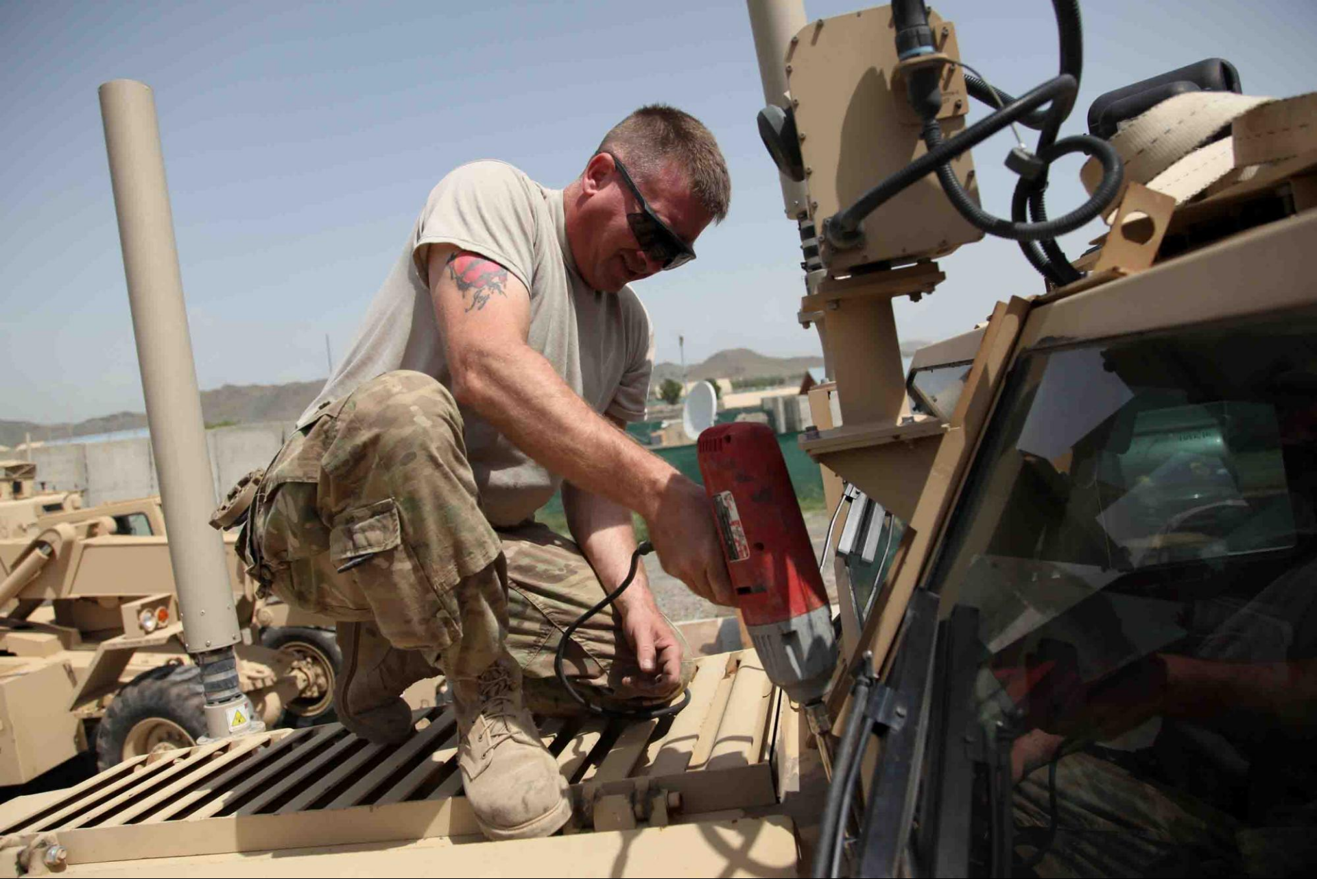
U.S. Navy Construction Mechanic 1st Class William Cook, attached to Provincial Reconstruction Team Khost, from Construction Battalion Maintenance Unit 202 Detachment Jacksonville, Fla., unbolts the windshield from a Cougar H 6x6 mine-resistant, ambush-protected vehicle on Forward Operating Base Salerno, Khost province, Afghanistan, Aug. 11, 2012. The windows periodically need replacing due to fogging between panes or cracks. (U.S. Army photo by Sgt. Kimberly Trumbull/Released)
