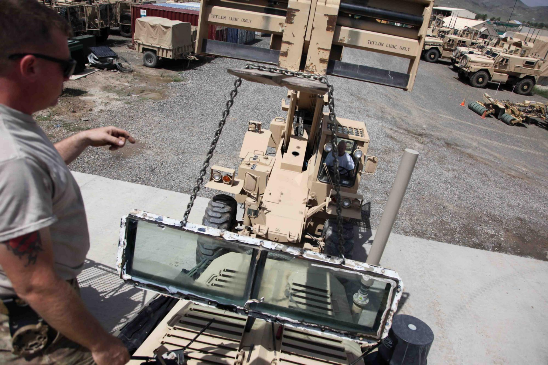
U.S. Navy Construction Mechanic 1st Class William Cook, attached to Provincial Reconstruction Team Khost, from Construction Battalion Maintenance Unit 202 Detachment Jacksonville, Fla., and Brian Coll, a force protection Cougar field service representative, use a forklift to remove the windshield of a Cougar H 6x6 mine-resistant, ambush-protected vehicle for replacement on Forward Operating Base Salerno, Khost province, Afghanistan, Aug. 11, 2012. The windows periodically need replacing due to fogging between panes or cracks. (U.S. Army photo by Sgt. Kimberly Trumbull/Released)
