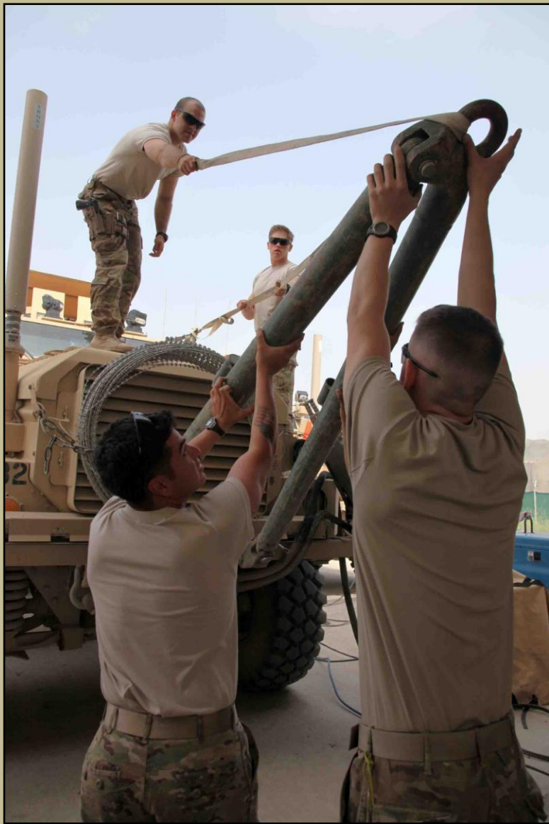
U.S. Soldiers, all combat infantryman with 1st Platoon, Delta Company, 1st Battalion (Airborne), 143rd Infantry Regiment, Task Force 4-25, lower a tow-bar to remove it from a mine-resistant, ambush-protected vehicle on Forward Operating Base Salerno, Khost province, Afghanistan, Aug. 10, 2012. U.S. Soldiers perform weekly maintenance on their vehicles to ensure mission readiness. (U.S. Army photo by Sgt. Kimberly Trumbull/Released)
