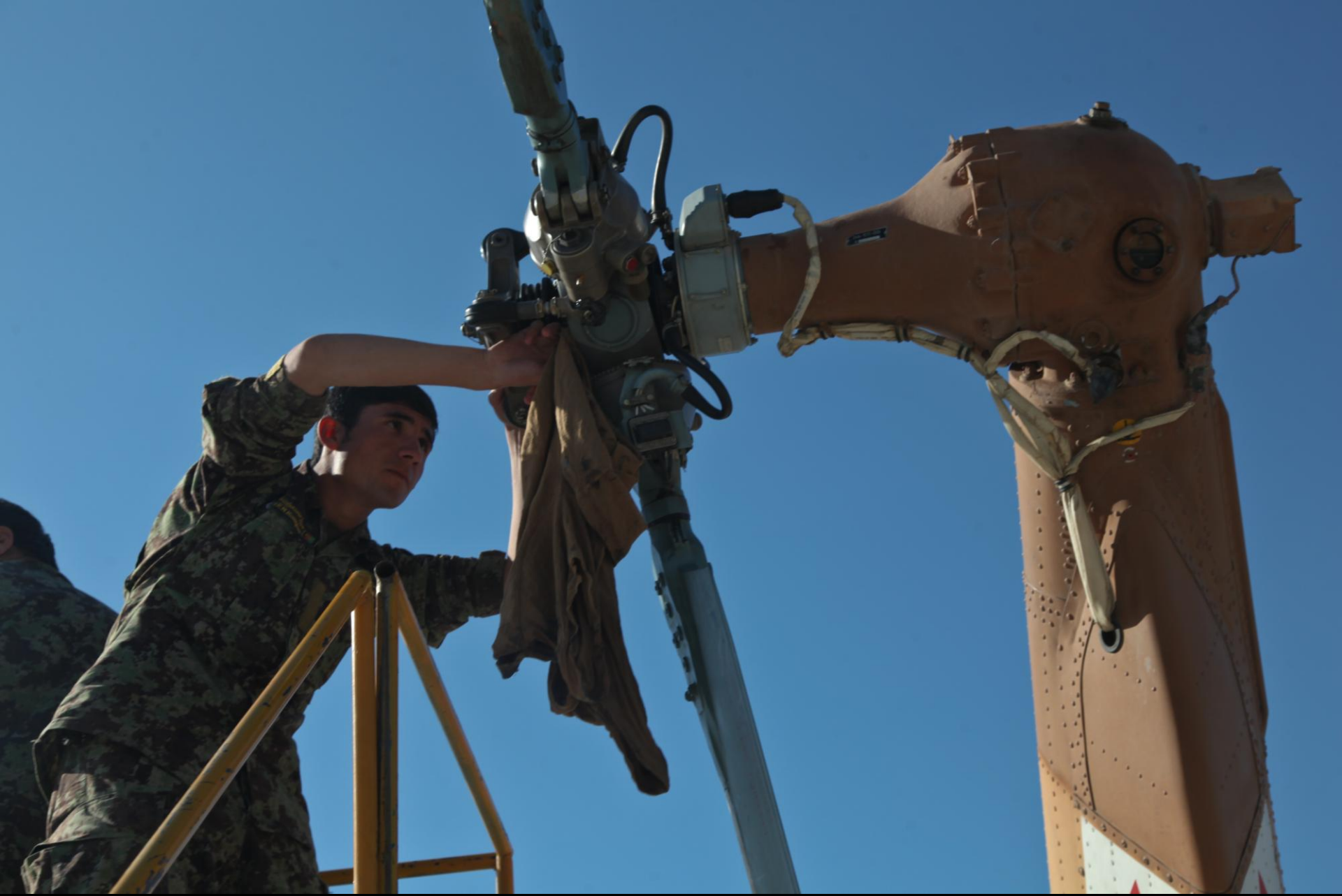
An Afghan National Army Air Corps soldier cleans the rear rotor of an Mi-17 Hip during aircraft maintenance at Forward Operating Base Fenty, Nangarhar province, Afghanistan, Nov. 19, 2012. Afghan National Army Air Corps soldiers prepare the aircraft to be utilized for a future joint mission. (U.S. Army photo by Spc. Ryan Hallgarth / Released)
