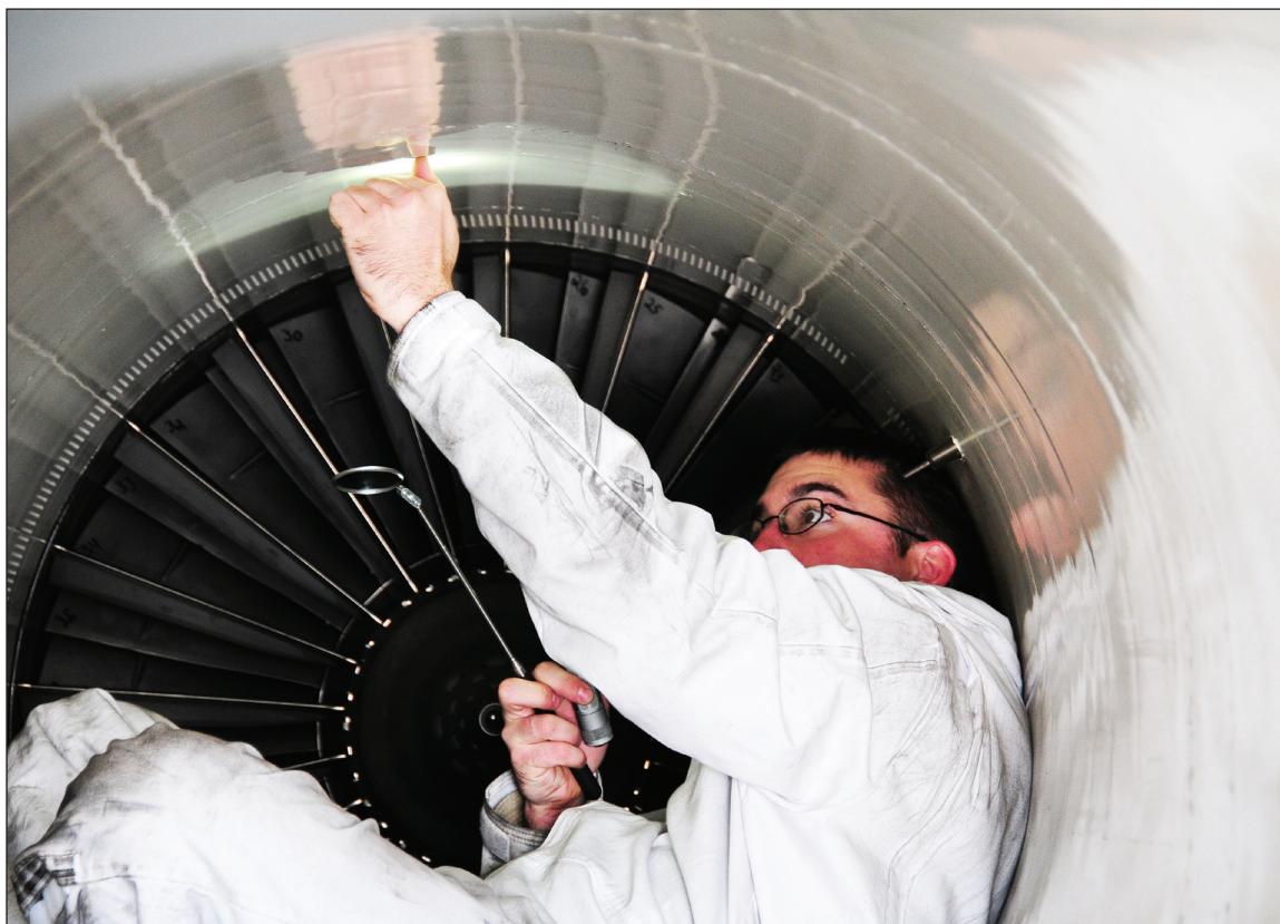
Air Force Staff Sgt. Brandon Deem, 44th Expeditionary Aircraft Maintenance Unit, inspects rivets in the No. 1 engine of an F-15C Eagle. Airmen, aircraft, and equipment from Kadena Air Base, Japan, are deployed to JBER supporting the Alaskan NORAD Region. (U.S. Air Force photo/Master Sgt. Mikal Canfield)
