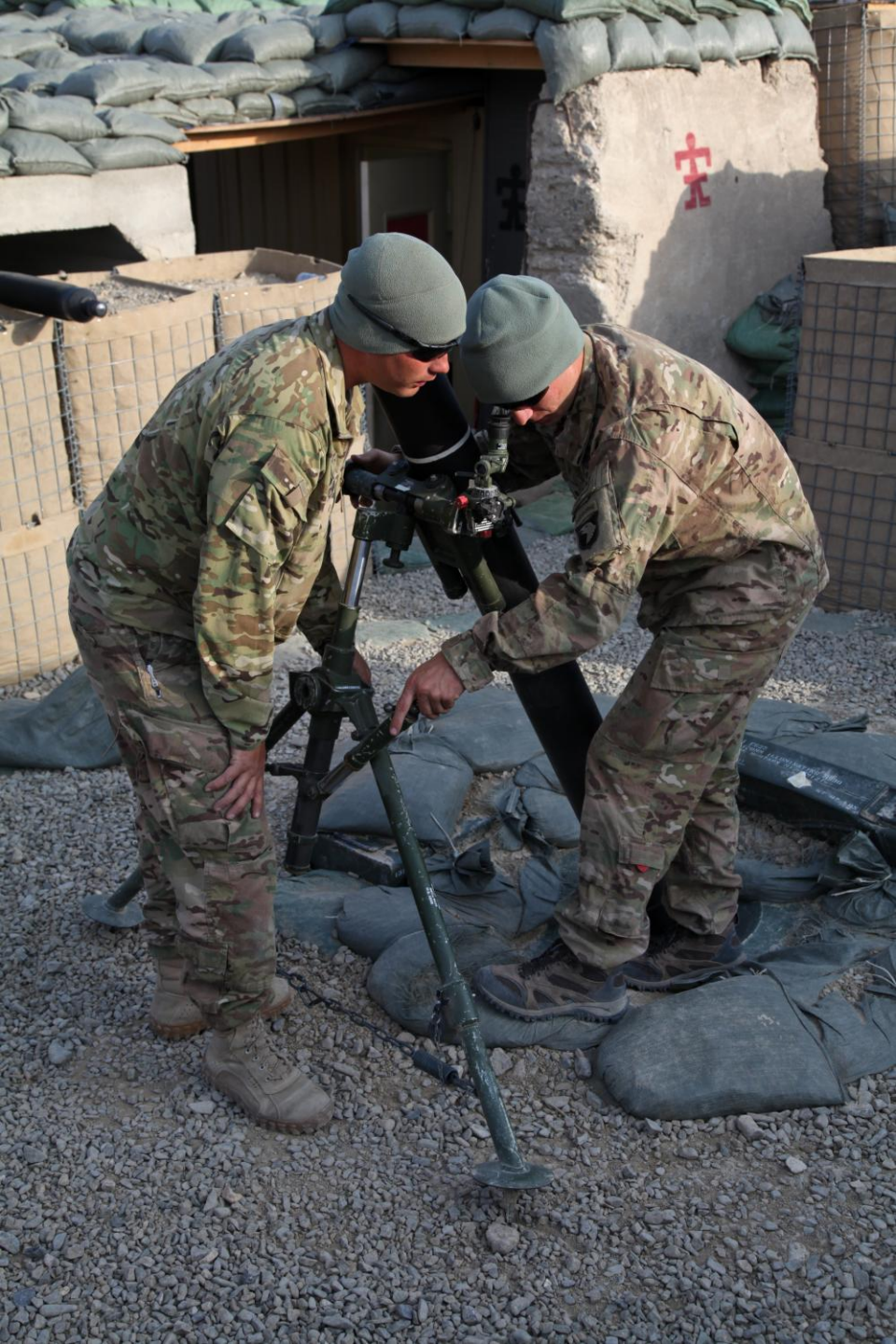
U.S. Army Spc. Craig Chambliss helps Spc. Timothy Reed, right, make a deflection change to a M120 120 mm mortar system on Combat Outpost Herrera, Paktia province, Afghanistan, Oct. 30, 2012. Both Soldiers, serving with 1st Battalion, 187th Infantry Regiment, 3rd Brigade Combat Team, 101st Airborne Division (Air Assault), were practicing for an upcoming gunner's exam. (U.S. Army photo by Spc. Jenny Lui/Released)
