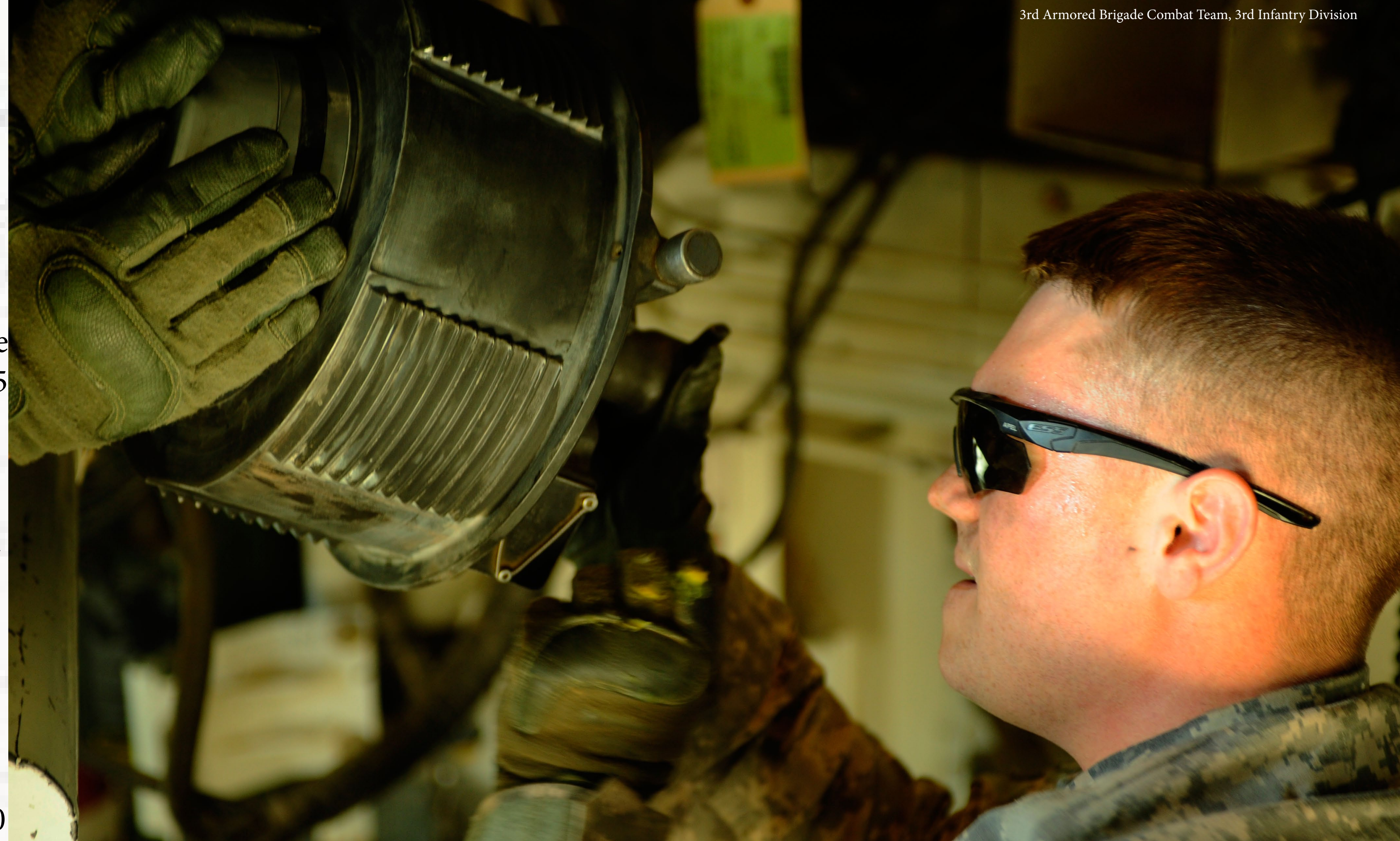
Spc. Kirk E. West, a cannon crewmember and Lancaster, Mo., native assigned to Alpha Battery, 1st Battalion, 10th Field Artillery Regiment, 3rd Armored Brigade Combat Team, 3rd Infantry Division, reassembles the breech of the 155 mm Howitzer inside his M109A6 Paladin during the 1-10 FA's Top Gun competition, Sept. 11 at Camp Buehring, Kuwait. Sixteen crews competed for the honor of Top Gun which showcased their knowledge and ability to perform multiple tasks within their Military Occupation Specialties. (U.S. Army photo by Sgt. Christopher Johnston, 3rd ABCT, 3rd ID Public Affairs)
