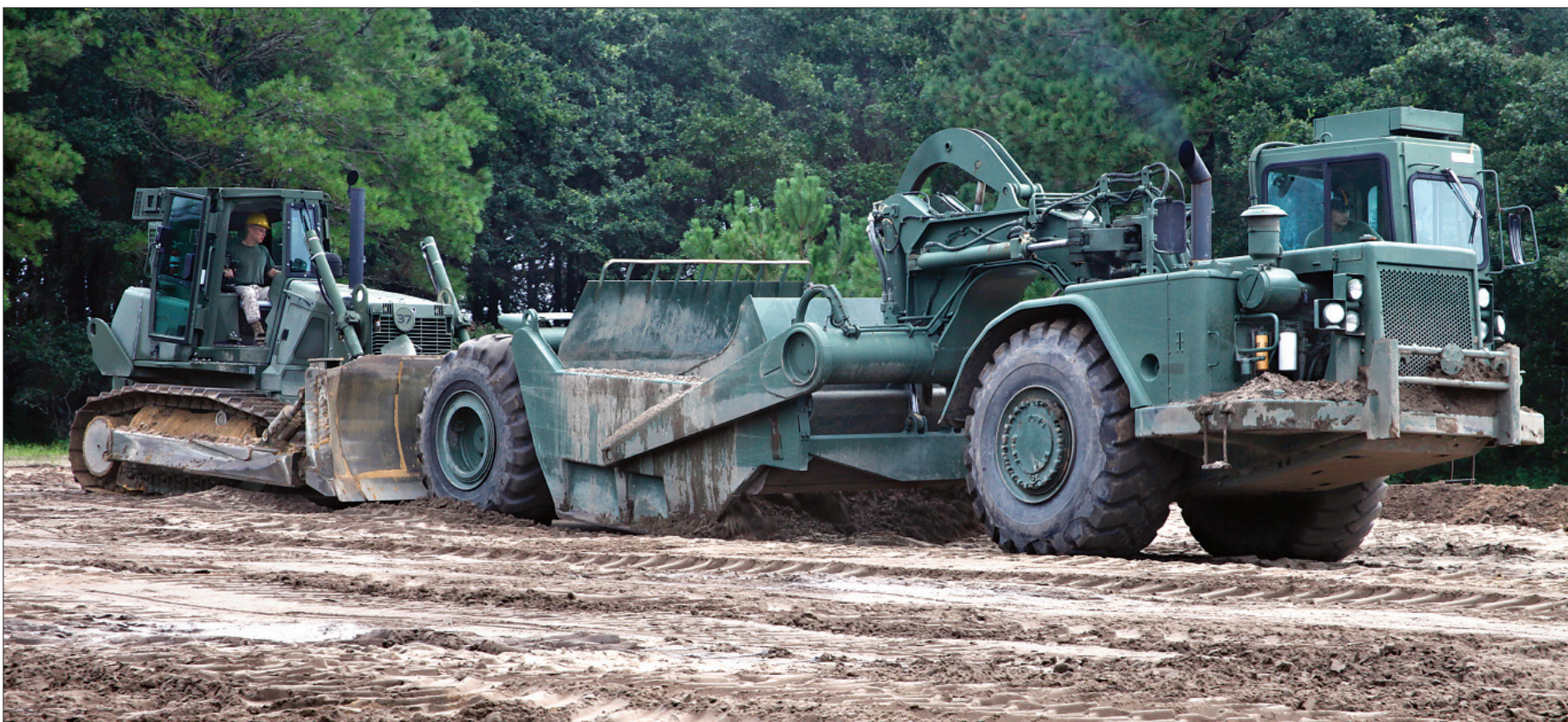
Marines from Marine Wing Support Squadron 274 use an 850 JR Bulldozer to assist a 621B Wheeled Tractor-Scraper to move dirt during a training class at Marine Corps Auxiliary Landing Field Bogue, N.C., Aug. 23. As part of the week-long course, the heavy equipment operators got hands-on with scrapers and other heavy machinery, equipment they don’t use on a daily basis.
