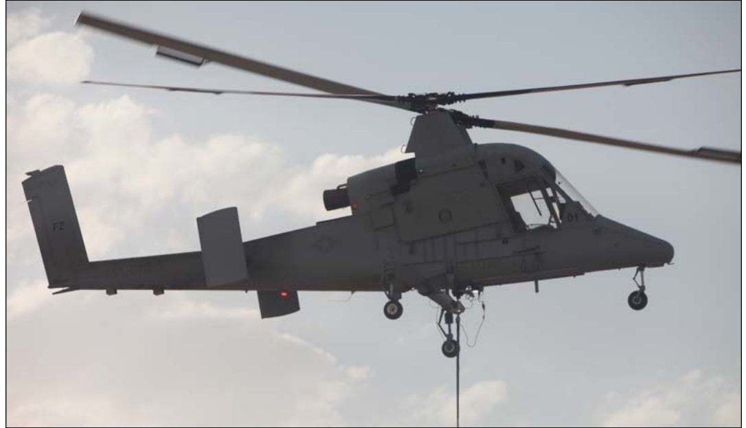
The Kaman K1200 unmanned aerial vehicle is a remote-controlled aircraft that is used to deliver supplies and gear to units in southern Helmand Province, Afghanistan. The aircraft can support up to 6,500 pounds and once in the air can independently pilot itself to a preprogrammed destination.
