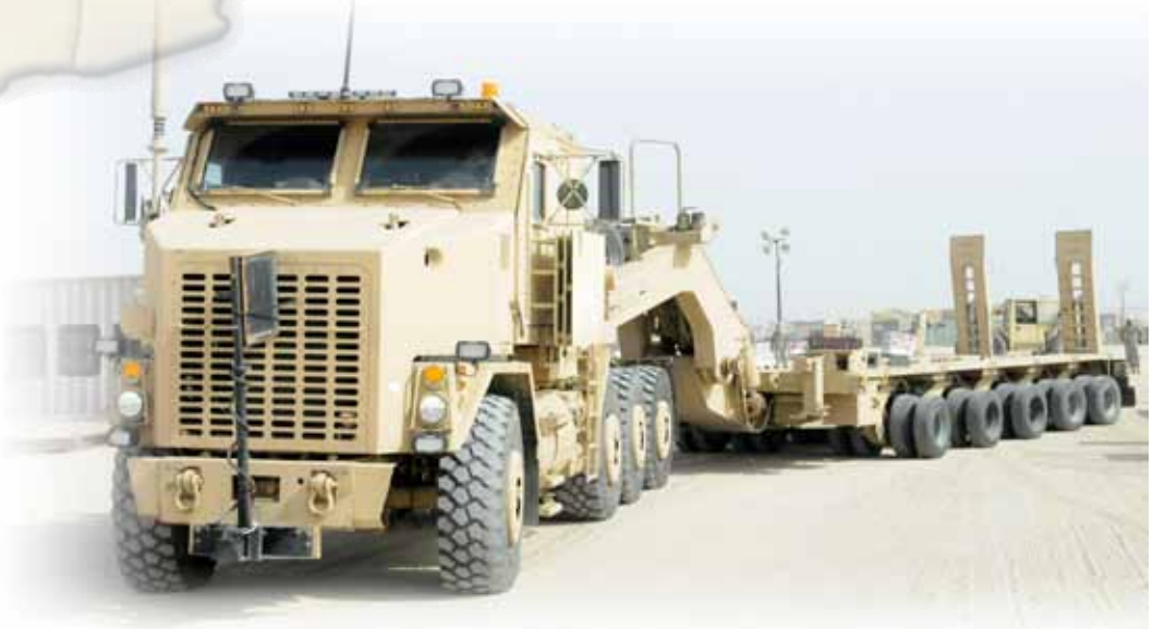
A Heavy Equipment Transport sits at Camp Arifjan's transportation lot in Zone 6, Feb. 10. HETs are used to transport, deploy and evacuate tanks, self-propelled artillery and other heavy vehicles and have served as a vital part of Third Army's mission in the drawdown of Iraq. Using HETS saves wear and tear on Mine Resistant Ambush Protected Vehicles and tanks, and is more cost efficient.
