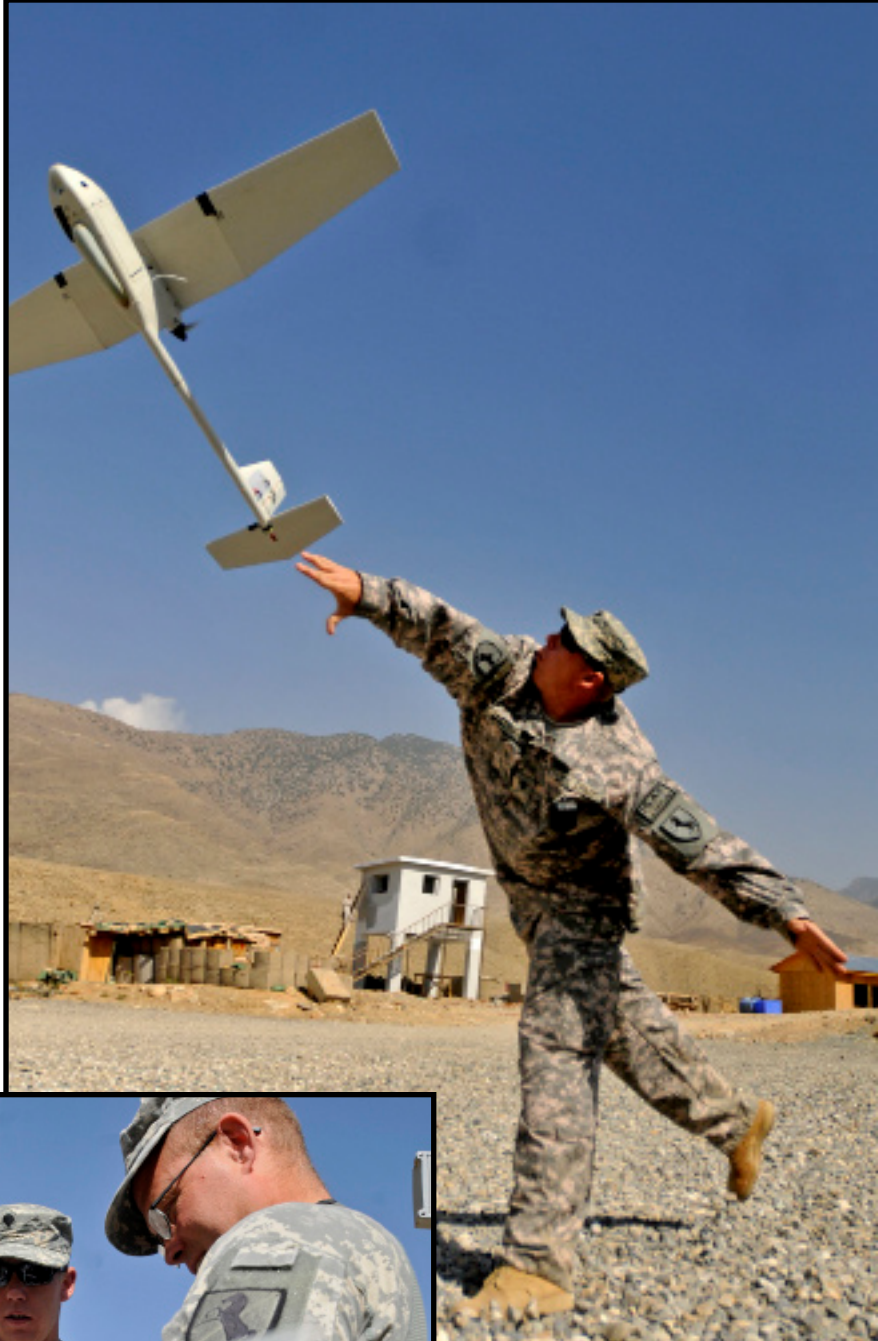
Above: Spc. Mitchell Matney, a Raven operator for Headquarters and Headquarters Troop, 1-221 CAV., and a Las Vegas native, launches a Raven unmanned aerial vehicle at Combat Outpost Nagil, Laghman province, Oct. 13. The Raven is able to provide real time video feeds once in the air.
