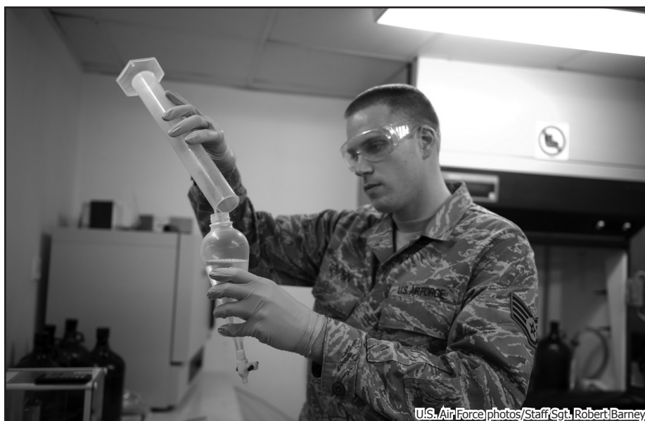
Staff Sgt. Damon Griffin, 379th Expeditionary Logistics Readiness Squadron fuels laboratory technician, tests a sample of JP-8 fuel, Wednesday, in Southwest Asia. The fuels laboratory ensures all fuel received meets Air Force standards from reception to its usage by local aircraft or ground vehicles. Sergeant Griffin is deployed from Ramstein Air Base, Germany, in support of operations Iraqi Freedom and Enduring Freedom.
