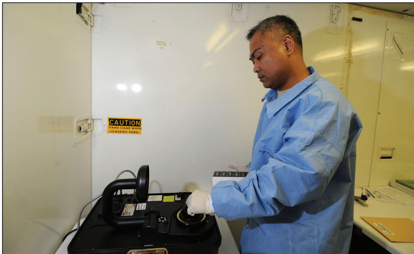
Maj. Lorenzo Gabiola, 379th Expeditionary Medical Group biological augmentation team chief, analyzes a simulated sample, Tuesday, using the base's new Joint Biological Agent Identification and Diagnostic System, which amplifies ribonucleic acid for H1N1 detection. Major Gabiola is deployed from Tinker Air Force Base, Okla. in support of operations Iraqi Freedom and Enduring Freedom.
