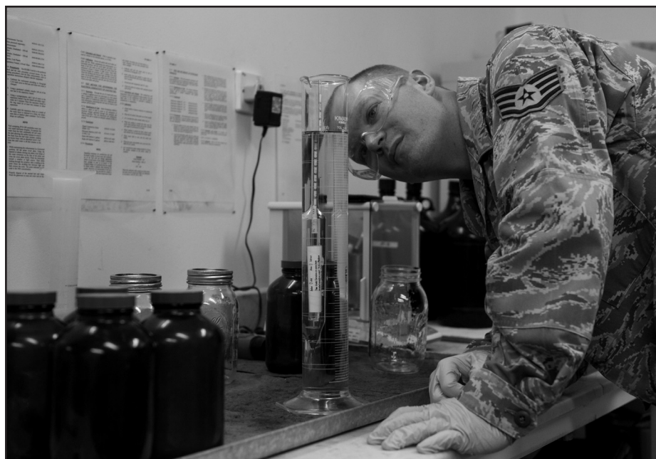
Staff Sgt. Michael Brady, 379th Expeditionary Logistics Readiness Squadron fuels laboratory NCOIC, performs an API gravity determination test on aviation gasoline, Wednesday, in Southwest Asia. Sergeant Brady is deployed from Dyess Air Force Base, Texas in support of operations Iraqi Freedom and Enduring Freedom.
