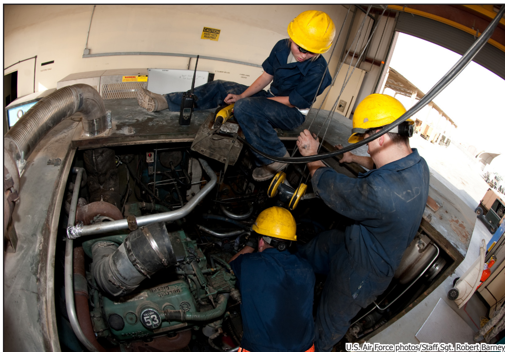
Clockwise from top, Airman 1st Class Kara Rouse, Staff Sgt. Donald Frazier and Senior Airman Kevin Desautels, 379th Expeditionary Maintenance Squadron aerospace ground equipment members, replace a main hydraulic pump on a hydraulic test stand, Wednesday, in Southwest Asia. The stand is used during B-1B Lancer maintenance. Airmen Rouse and Desautels are deployed from Ellsworth Air Force Base, S.D. and Sergeant Frazier is deployed from Dyess AFB, Texas, in support of operations Iraqi Freedom and Enduring Freedom.
