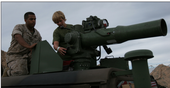
Corporal Andrew C. Hanson, an anti-tank missileman with Weapons Company, 1st Battalion, 1st Marine Regiment, 1st Marine Division, shows Chris, 12, from San Diego, the M-220 Tube launched, Optically tracked, Wire-guided (TOW) missile weapon system as part of a static display at the MCAS Miramar Air Show, Oct. 2.
