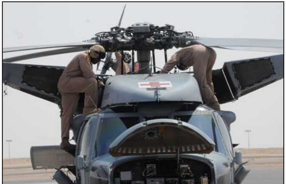
2515th Naval Air Ambulance Detachment maintainers, conduct a preflight inspection on a MH-60S Helicopter.
